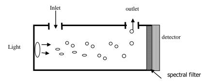
Basic mathematical model: A majority of both organic and inorganic polyatomic gas have specific absorptive wavelength in infrared region. It observes Lambert-Beer Law formula I=I0e-kpl when infrared light is coming through. Light absorption intensity "i" can be described as i=I0-I= I0 (1- e-kpl). I0: intensity of incoming ray. I: transmitting beams. I :thickness of gaseous medium. p: gas concentration. k: absorption coefficient.
